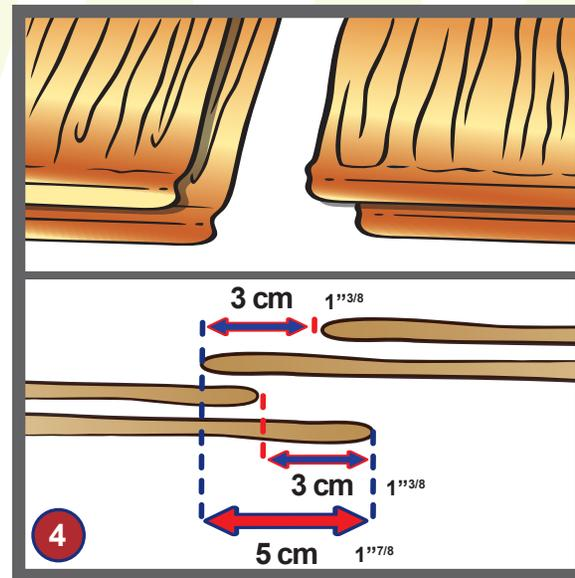
4) For the first two rows: insert a double layer of leaves with a 3 cm (1" 1/4) overlap on the rail.
