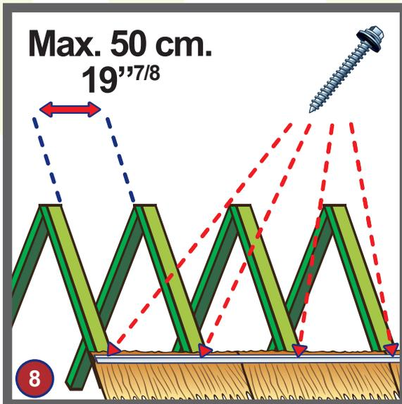
8) Fix rails to vertical battens. Space between battens must be a maximum of 50 cm (19" 5/8).
