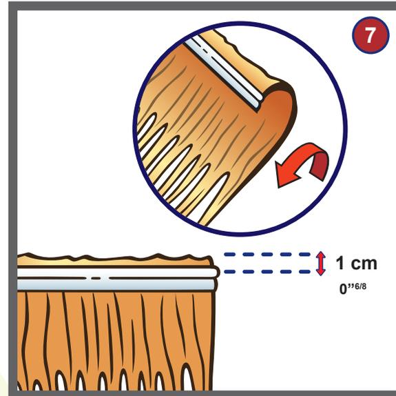
7) Before fixing rails, fold the rounded part of the leaves down in order to get a minimum of 1 cm (0" 1/2) space between the rail and the folded part of the leaf.
