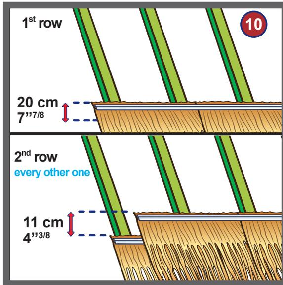
10) Fix the first rail with leaves at 20 cm (7<sup>7/8</sup>) from the bottom of the roof and 11 cm (4<sup>3/8</sup>) for every other one from the last one.
