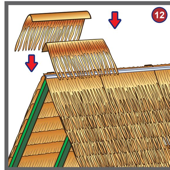
12) For extra protection against water infiltration and for aesthetic reasons, add our patented Palmex ridge or add another row of leaves at both ends (and on both sides) on the very top of the roof, extending 11 cm (4<sup>3/8</sup>) on either side of the roof (both sides must first be finished).
